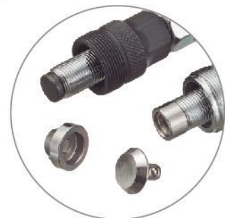
ST- 241C,D For Shimano Octalink and ISIS Drive system. Threaded nut includes smoothed ring at head to prevent damage to thread.
